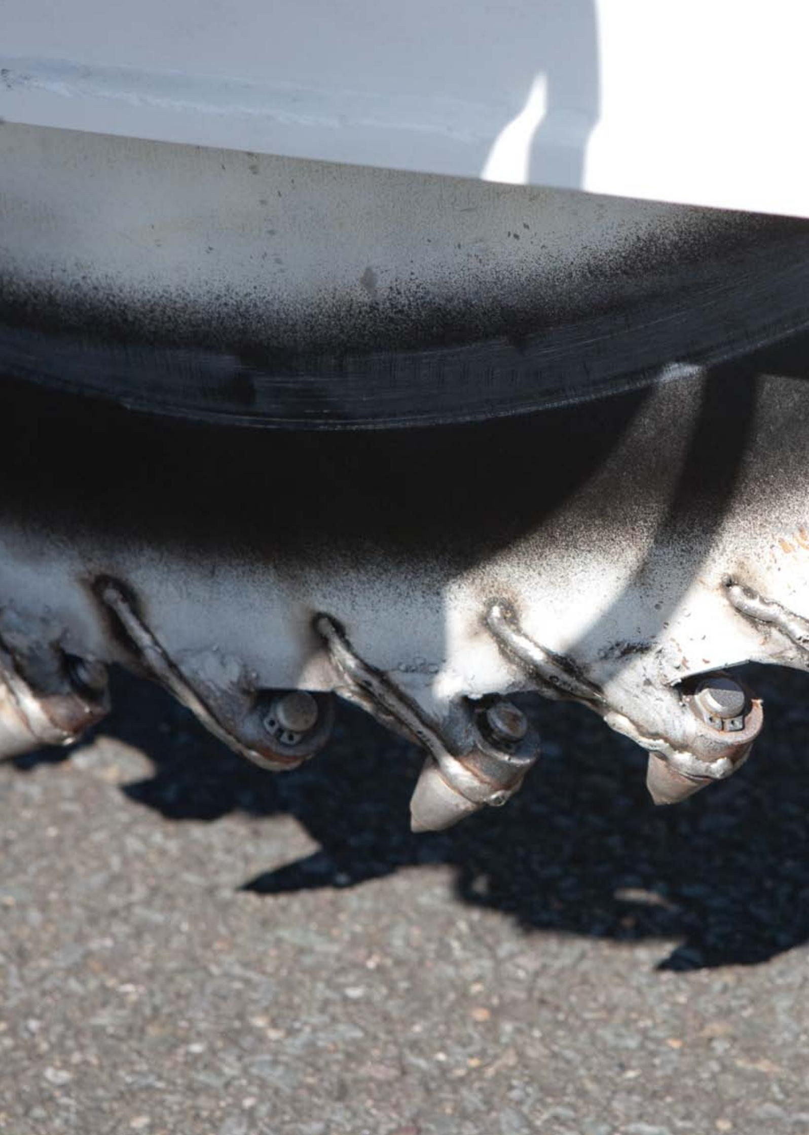
**LEFT** The teeth of Marais Lucas' Sidecut microtrencher, about to bite into an international airport's tarmac to install new lighting cables. Our Cleanfast and Sidecut machines were ideal for this project, which needed to be completed, ready for aircraft traffic, during the airport's night-time curfew. Speed, safety and flexibility make these ideal for installation of power, telecommunications, gas and water pipelines and conduits.
